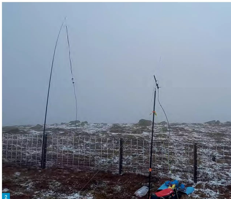
Fig. 1: Keith G4ITR prepares the 11 element yagi that he and Graeme M0EUK used during the 145 Alive event from the North Pennines.
