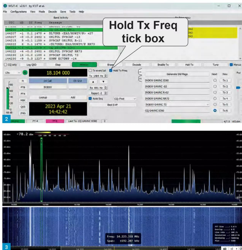
Fig. 1: WSJT-X FT4 Wide graph display. Fig. 2: WSJT-X Hold Tx Freq check box. Fig. 3: Receiver spectrum display (SDR Console). Fig. 4: FFT bins. Fig. 5: Hamming window shape. Fig. 6: Using SDR# Studio to display the FT8 band activity. Fig. 7: Slow speed waterfall showing 20m activity. Fig. 8: High-speed waterfall reveals Morse code.
